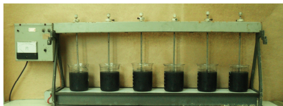
Figure 1. Jar-Test equipment used during the study.
