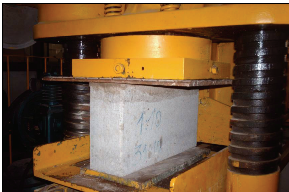
Figure 3. Compressive strength test.
