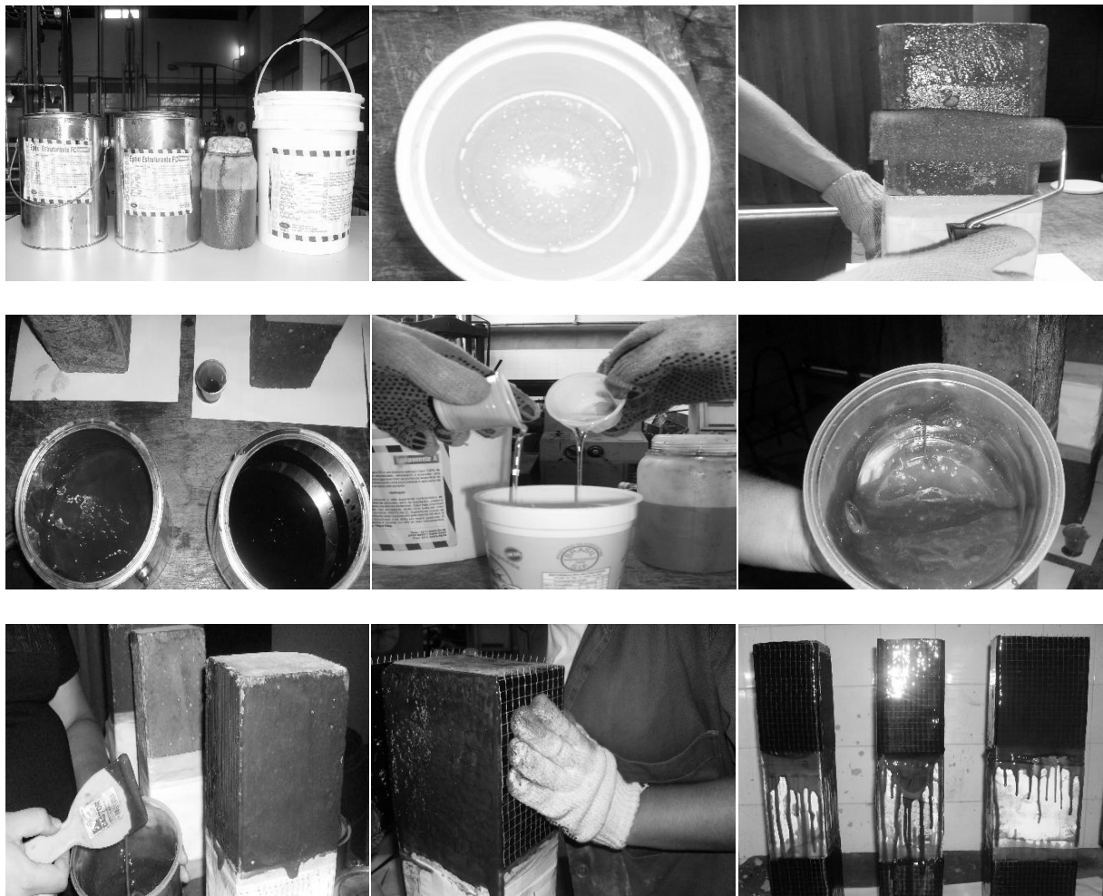
Figure 5. Step-by-step process to strengthen the short columns.
