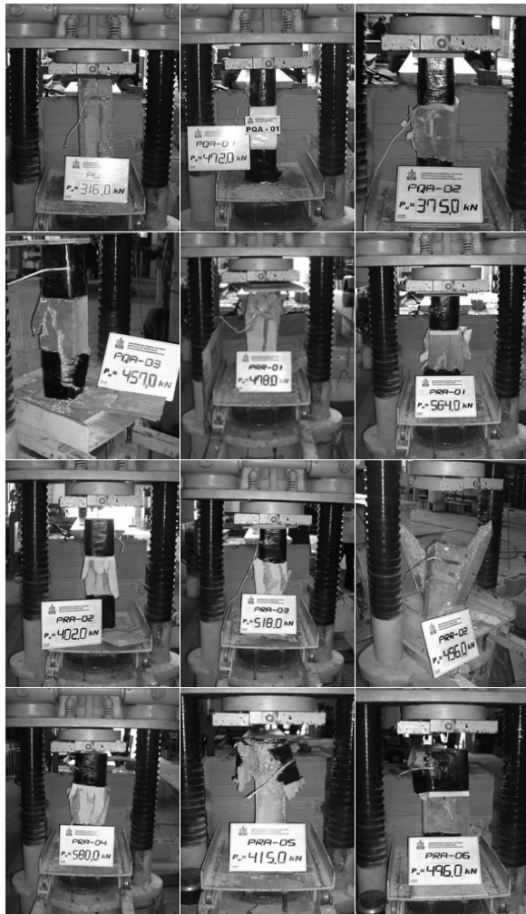
Figure 6. View of columns after tests.
