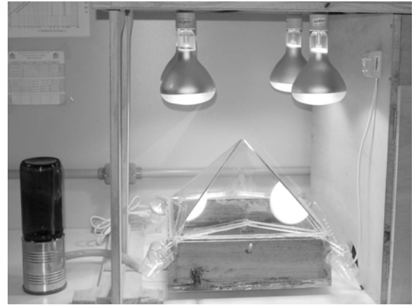
Figure 3. Pilot for determining the best water level on the evaporation pan for inclination at 45°
