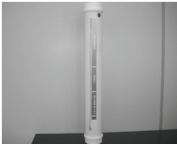
Figure 11. Detail of timer scale for one and half hour irrigation.
