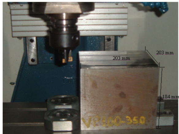
Figure 1. Block VP 100 used in the tests milling mounted on the table of the machining center.
