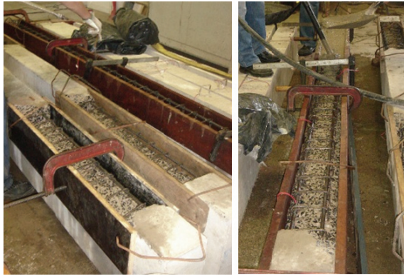
Figure 5. Removal and reconstitution of the tensile zone of the beams of the groups C and D.
