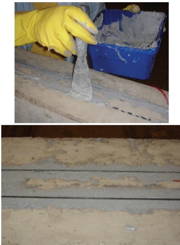
Figure 6. Procedures to apply the strengthening on the tensile zone of the beams.
