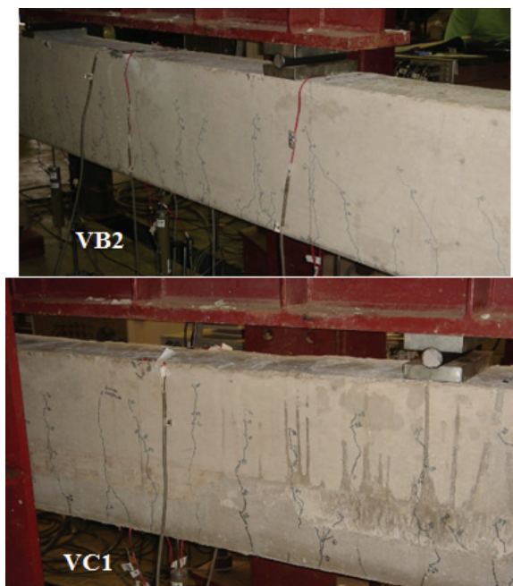
Figure 8. Cracking in the beams of the group B and C.
