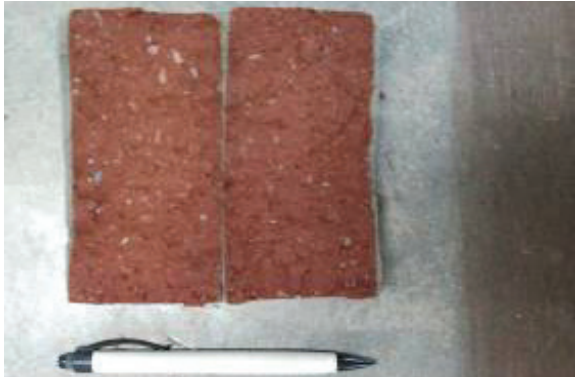
Figure 4. Sample inner aspect after failure.
