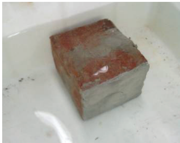
Figure 2. Specimen immersed in water before performing compressive strength.
