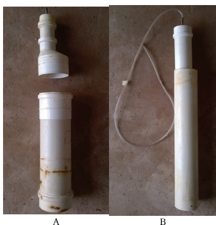
Figure 2. Reactor model (A); gasometer model (B).
