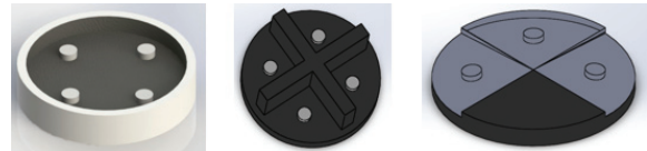
Figure 1. Light sensor designs (a) lateral trim (b) central side trim and (c) with different slopes in the sensor planes.
