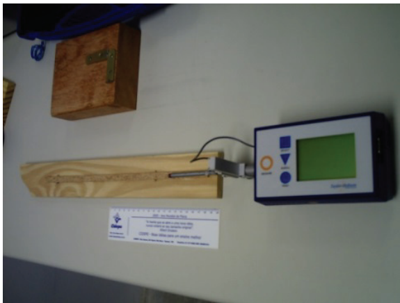
Figure 4. Rugosimeter device to verify roughness of PHPM.
