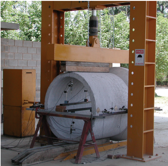
Figure 3. View of the diametrical compression test.
