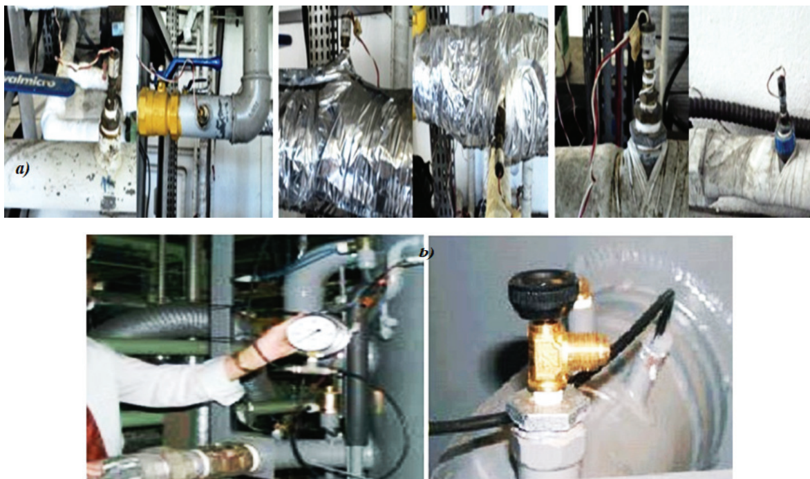
Figure 4. a) Temperature measurement point of the external water circuits, used in the microgeneration laboratory (cold, hot and chilled water, respectively). b) Pressure reading socket used to measure the mass flow water rate and pressure difference of the water circuits (Yazaki Energy System, 2003).
