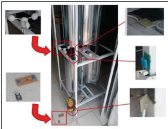
Figure 5. Position of the controller board and the sensor on structure of the turbine.
