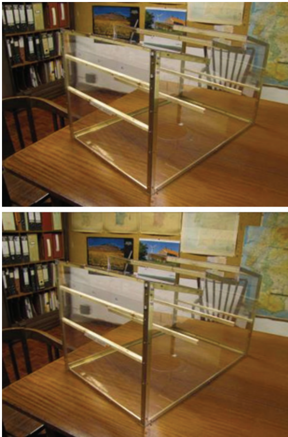
Figure 2. The reduced-scale model tested in wind tunnel.
