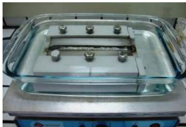
Figure 5. Plate welded by MIG/MAG process, immersed in NaCl.
