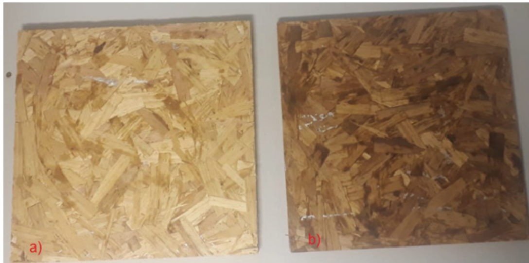
Figure 1. a) Control treatment board; b) Heat treated board.
