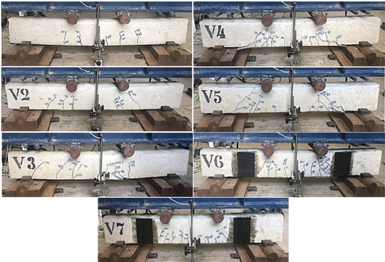
Figure 6. Beams after failure. Source: Author.
