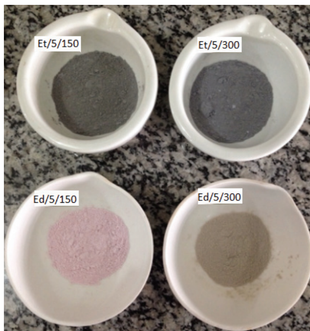
Figure 6. Co/SBA-15 catalysts after leaching and heat treatment.
