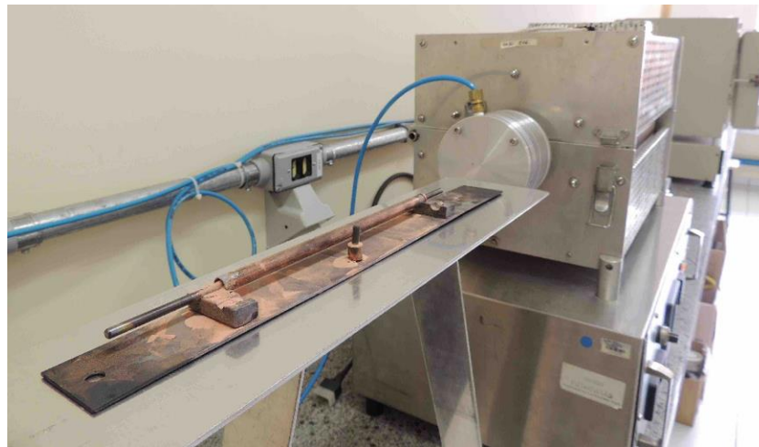
Figure 5. Preparation of the heat pipe for sintering process.
