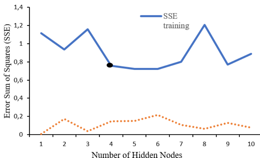
Figure 2. Graph of error sum of squares (SSE) against number of hidden nodes in ANN hidden layer – ANN models using significant variables from bivariate linear regression analysis as factor. Straight line represent errors from training subset and dotted line represents error from testing subset. Best model is represented by a dot.
