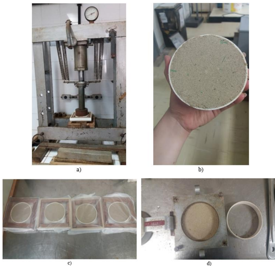
Figure 5. Molding of specimens for direct shear tests: a) static molding of the specimen; b) specimen molded in the ring; c) curing of specimens; d) specimen transferred to the shear box after 7 curing days.
