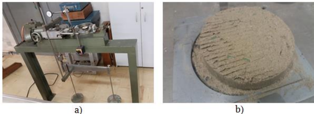
Figure 6. Direct shear test: a) equipment used; b) specimen after test.
