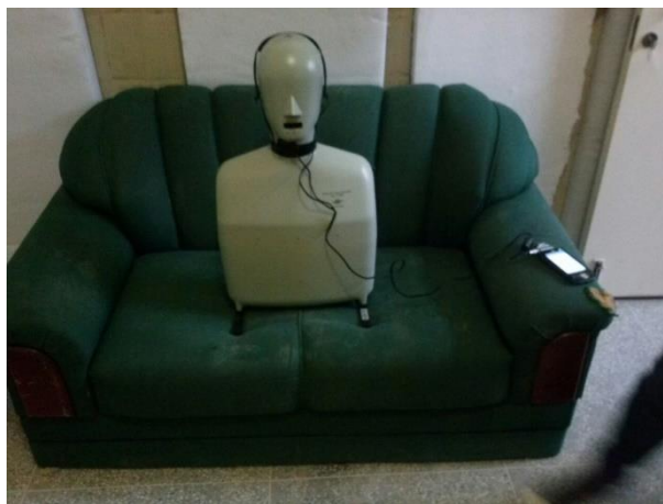
Figure 4. Assembly of the recording equipment in the adapted receiving room of the impact chamber.
