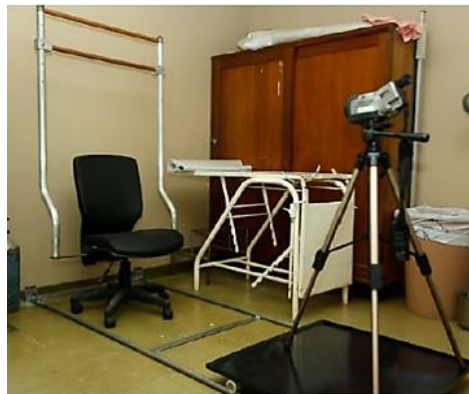
Figure 2. Mechanical apparatus used in the thermographic image capture protocol.
