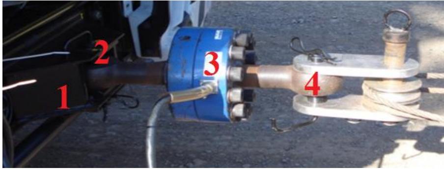
Figure 7. Load used in the experimental tests: (1) Body base plate; (2) Hitch pin; (3) Load cell; (4) Load.
