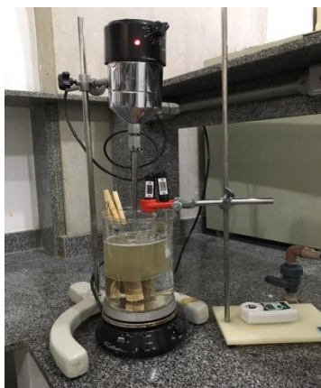
Figure 1. Assembly of the equipment used in production of gels inside a 1 L Beaker supported by cork stoppers inside a 2 L Beaker containing ethylene glycol solution at 40%, coupled on a heating plate, and to a mechanical stirrer.
