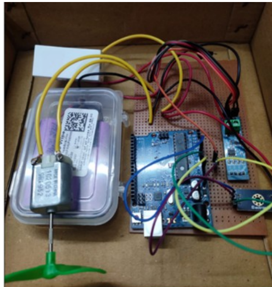
Figure 10. Hardware model of optimal charging system for dynamic wireless power transfer of EV.
