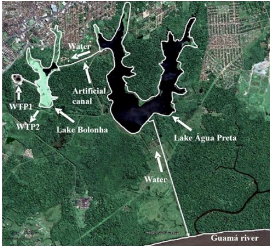
Figure 1. Water circuit in the Utinga system from collection in the Guamá River to outlets for treatment plants.
