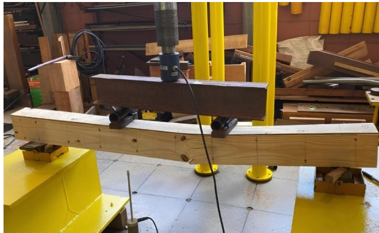
Figure 11. Predominant failure mode for NLT beams in bending. Own authorship.
