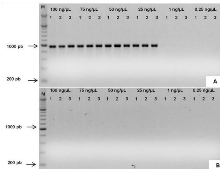
**Figure 2.** PCR reaction in 1% agarose gel electrophoresis using DNA from the IBSBF 278 (*Xanthomonas phaeoli* pv. *manihotis*) isolate in different concentrations, in the following order: 100, 75, 50, 25, 1, and 0.25 ng with three replicates each (1, 2, and 3). A: Reaction with primers XV/XK\_MOD; B: Reaction with primers XV/XK (Verdier et al., 1998). M: 200 bp DNA ladder.
