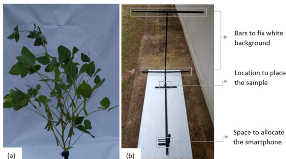
Figure 1. Image captured from pods of a single plant with image acquisition method 1 (IA1) (a). The frame used for sample positioning with image acquisition method 1 (IA1) (b).
