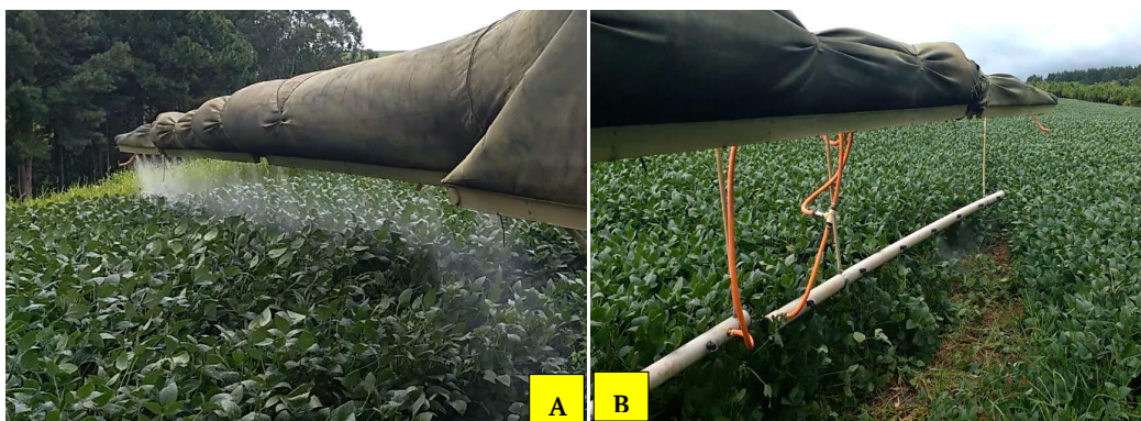
Figure 1. Boom with air-assist technology sprayer (A - Vortex™) and auxiliary boom (B - Kit Alvo™) designed for spraying pesticides in order to improve the penetration of drops in the leaf canopy.
