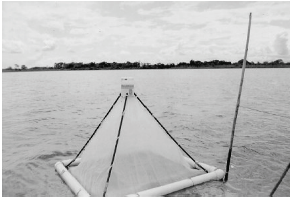
Figure 2. Model of floating emergence trap for capturing adult insects.
