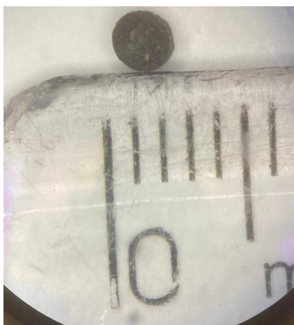
Figure 1. Illustrative image of PE scaffold, manufactured by the PE extracted from the marine sponge Aplysina fulva .
