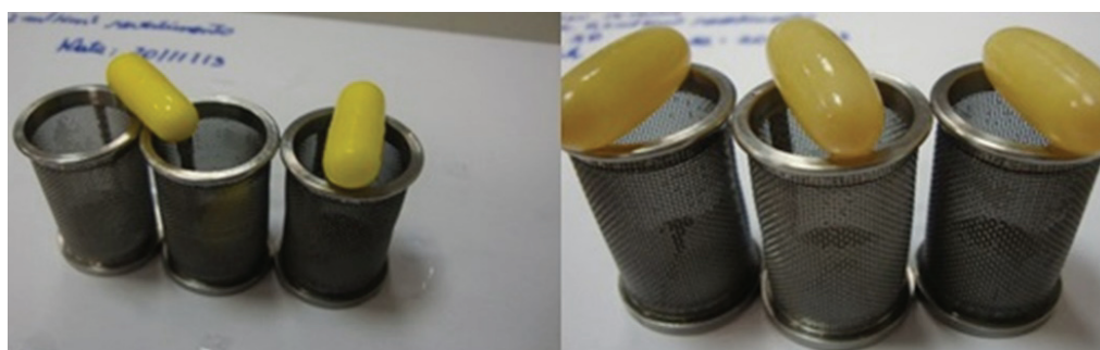
Figure 5. Glutamine and palm oil capsules coated with 0.2 mL of 6.5% Eudragit cm -2 after the second stage of disintegration in phosphate buffer at pH 6.0, with a test time of 3 hours.
