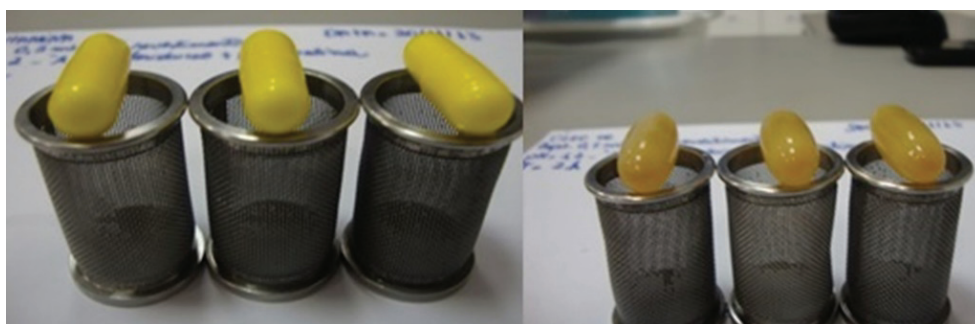
Figure 4. Glutamine and palm oil capsules coated with 0.2 mL of 6.5% Eudragit cm -2 from the first stage of disintegration in hydrochloric acid (pH = 1.2), with a test time of 2 hours.
