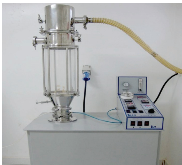
Figure 1. Spouted bed (Labmaq®, Ribeirão Preto, São Paulo, Brazil) used to coat the palm oil and glutamine capsules, purchased by the Gastrointestinal Surgery Department – UFTM.
