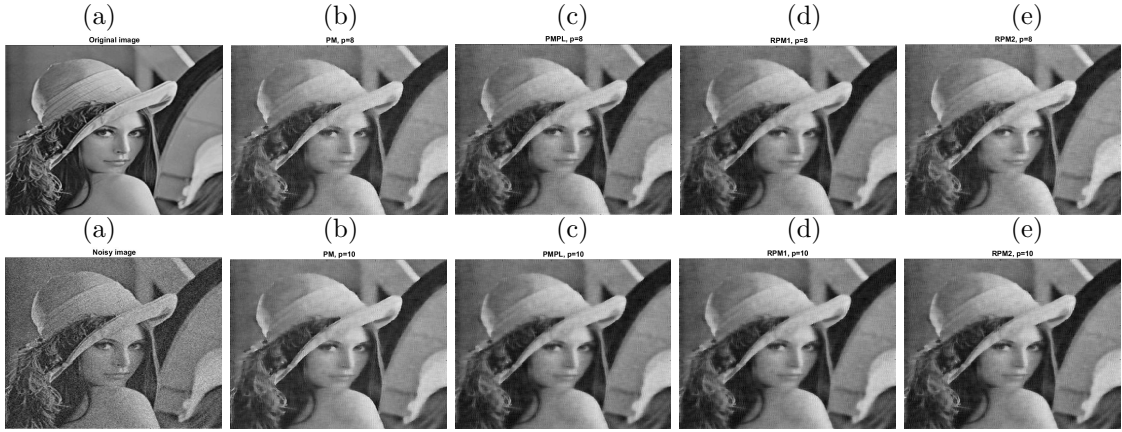
Figure 2: Compare the restored images using the different following models: (a) the initial and noisy images, (b) the PM filter, (c) the PMPL filter, (d) the RPM1 filter and (e) the RPM2 filter, with a fixed parameter \lambda = 10 and p changed.
