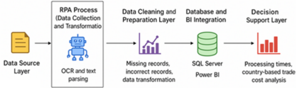
Figure 1: RPA-Based data flow diagram
