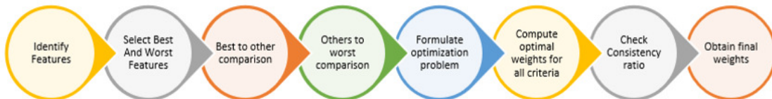
Figure 3: Steps to obtain weights by using BWM
