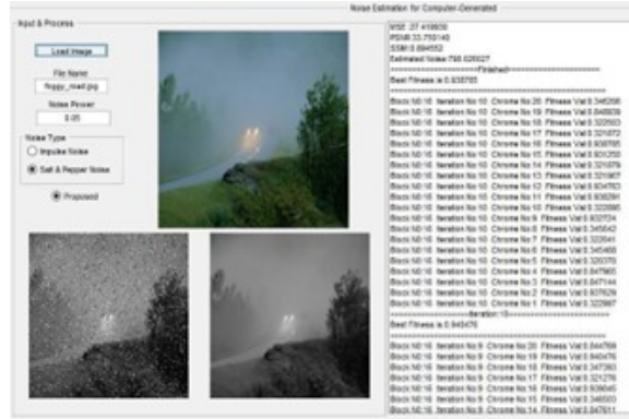
Figure 5: Noise estimation at noise power 0.2
