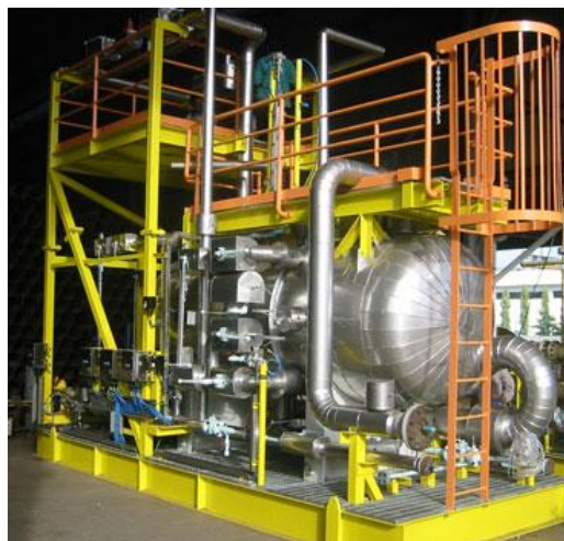
Figure 1: WWTP used on oil rigs. Credits: Veolia Water Technologies & Solutions
