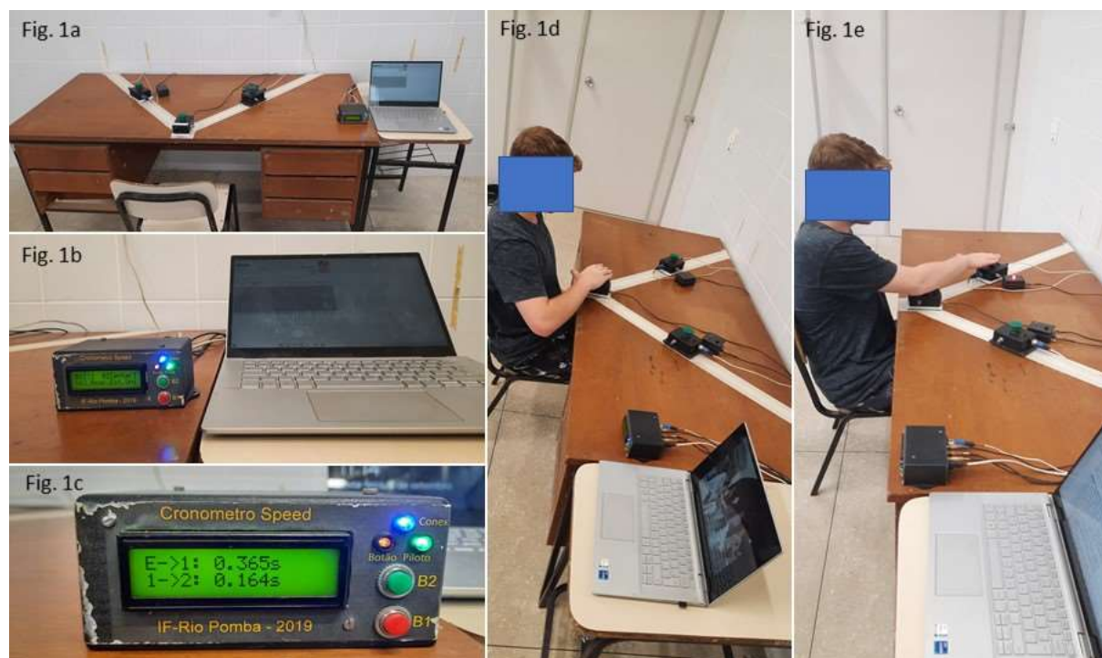
Figure 1. SPEED Equipment. 1a: Arrangement of buttons on the Speed equipment; 1b: LCD
