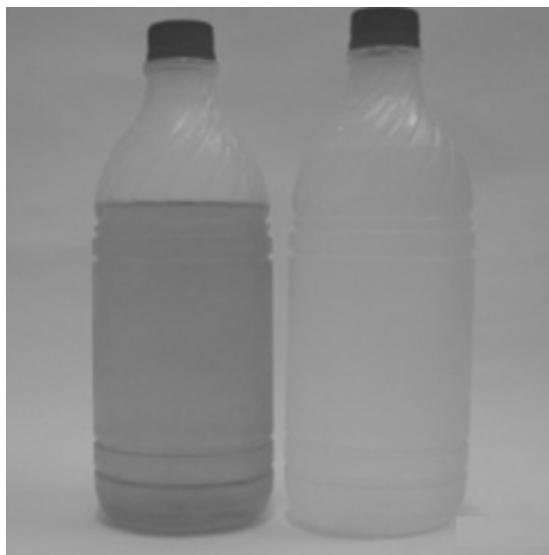
Figure 9. Comparison between the incoming water (left) and output (right) of the desalinator.
