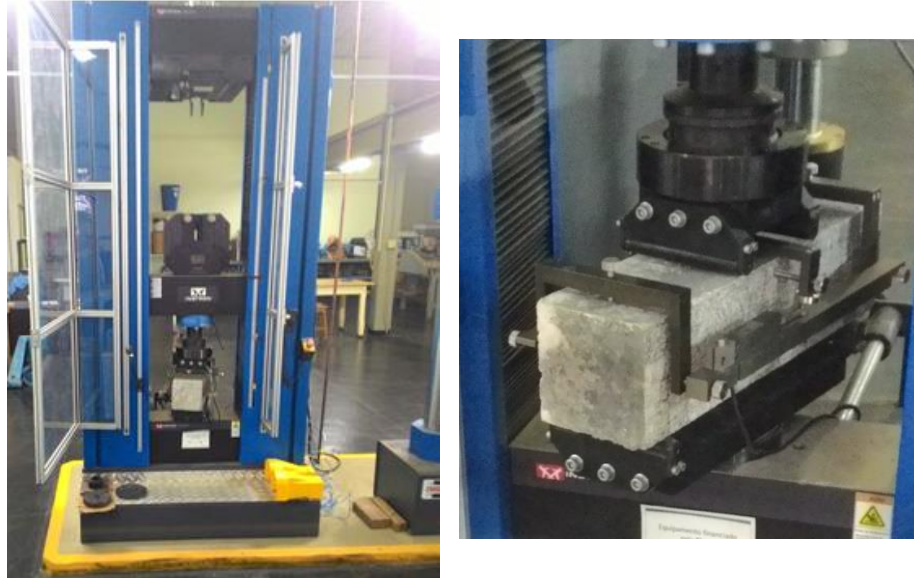
Figure 4. Specimen positioned in universal testing machine.
