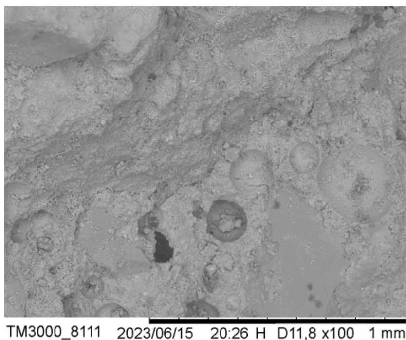
Figure 3. SEM image with 100x magnification of the broken concrete sample
