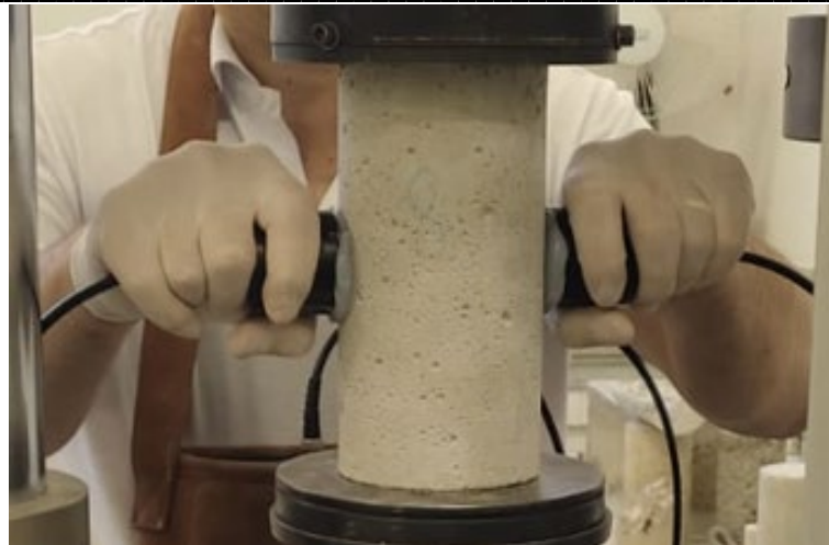
Figure 1. Measurement of UPV in the radial direction of the specimen
